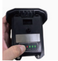
Battery indicator light
