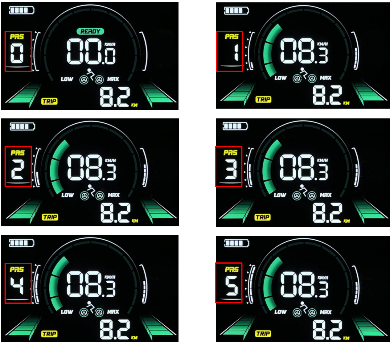
Figure 5-5: Level Switch Display
