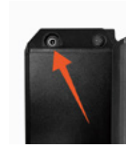
Battery Charging Port
